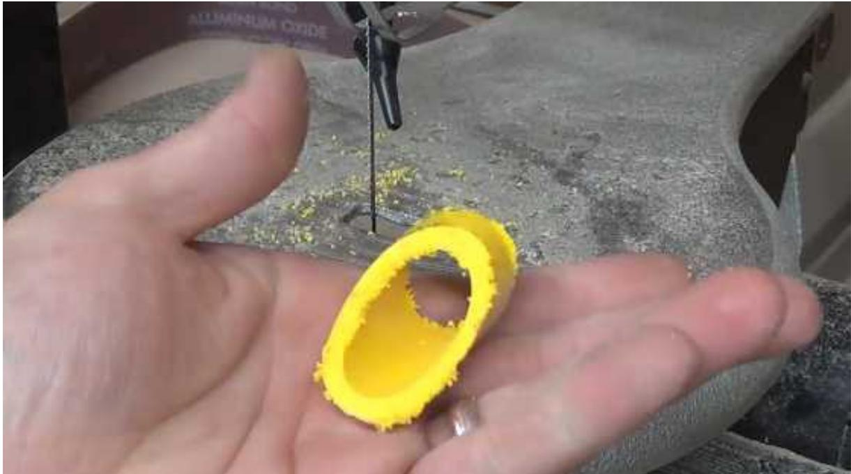
cut the pipe at an angle
